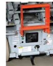
Charger at rear of base
