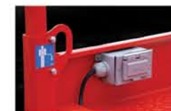
110V GFI AC protected outlet to platform and lanyard attachment point
