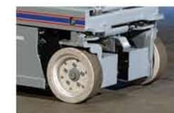
Compacts feature variable speed front wheel hydraulic drive
