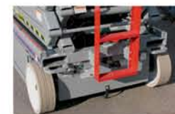
Forklift pockets and tie downs/lift lugs
