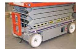
Conventionals feature variable speed rear wheel hydraulic drive
