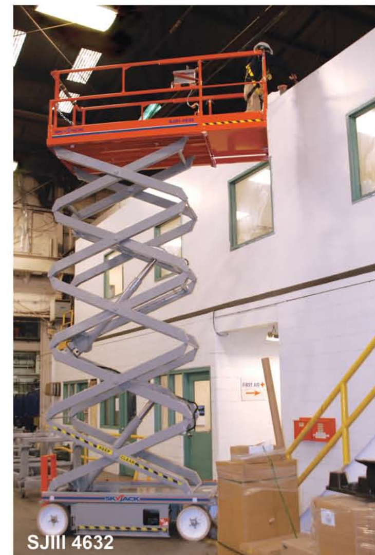
Conventionals feature variable speed rear wheel hydraulic drive
